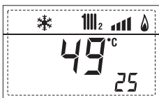
24. Visualisation safety thermostat with board ZONA MIX 2 (input S1) respectively ON and OFF
