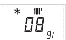
35. Software version on EXP (configuration ZONA MIX)
